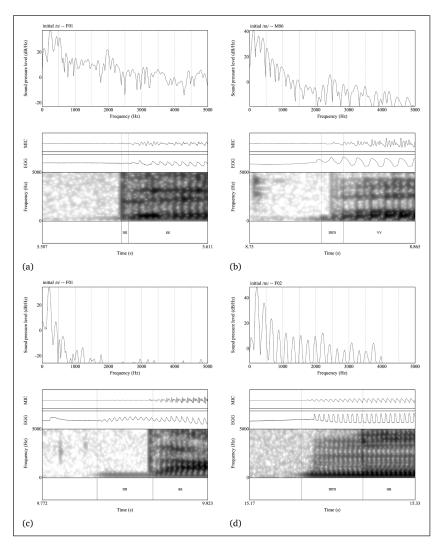
**Figure 4:** From top to bottom: FFT spectrum at nasal midpoint in phrase-initial position using a 30 ms Gaussian window, waveform, EGG signal, spectrogram of the acoustic waveform. (Amplitude scale: [-1, 1]; dynamic range: 60 dB). **(a)** Devoiced (speaker F01); **(b)** Prevoiced with short voice lead (speaker M06); **(c)** Prevoiced with no audible nasality (speaker F01); **(d)** Plain nasal (speaker F02). (Intensity and spectral analyses were excluded for (a) and (b)).
